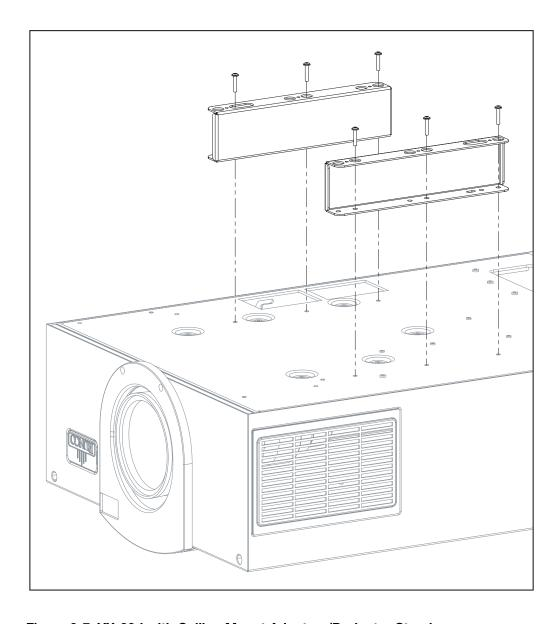
Figure 3-7. VX-33d with Ceiling Mount Adapters/Projector Stands
